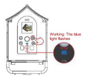
Select the "function icon, and click the button to enter recording mode. At this point, the feeder will automatically turn off the display. When birds or objects enter the PIR sensing area, the indicator light will flash blue, and the feeder will start recording. The camera will automatically record 10s/30s/1 minute/3 minutes of video without manual operation.
