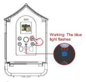
the button to enter camera mode. The feeder will automatically turn off the display when birds or objects enter the PIR sensing area, and the indicator light will flash blue. The camera will automatically take 3/5/10 pictures without manual operation.
