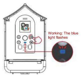
Select the "Function icon, and click the button to enter the camera+video mode. At this point, the feeder will automatically turn off the display. When birds or objects enter the PIR infrared sensing area, the indicator light will flash blue, and the feeder starts to work. The camera of the bird feeder will automatically capture 3/5/10 photos first, and then take a 10s/30s/1min/3min video without manual operation.
