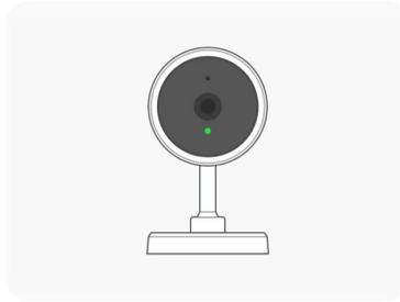
Power on the device and make sure the indicator is flashing rapidly or a prompt tone is heard.
