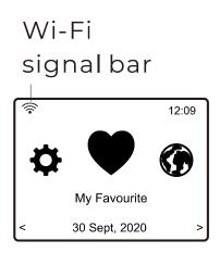
When the Wi-Fi connection is successful, the Connection Complete will be shown briefly. The Wi-Fi signal bar will appear in the top left corner of the display:
