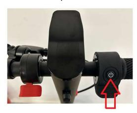
When scooter display is on you press one time on power button and light is on or off.
