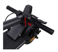
3) Close the lock lever located on the lower part of the handlebar support tube.
