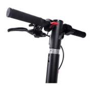
2). After matching the holes in the handlebar with those of the frame, insert the screws and tighten them well. Repeat the operation also in the side opposite side of the handlebar. All 4 screws should be used.
