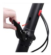
2. Fully open the release lever.
