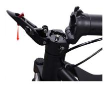
4. Hook the folded tube onto the appropriate support.
