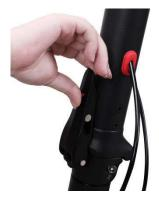
4) The electric scooter is unfolded as soon as you hear the rod clicks into place.
