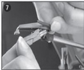
separate the cartridge from the socket lightly.
