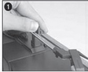
push the arm lock to release the tone arm.
