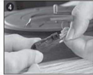
take off the audio lines from the cartridge completely.
