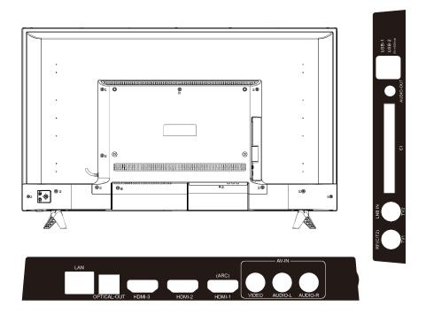
LAN(RJ45): RJ45 plug for connecting to external modem or network access equipment.
