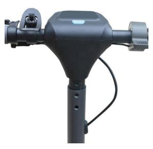
2). After matching the holes in the handlebar with those of the frame, insert the screws and tighten them well; repeat the operation also in the side opposite of the handlebar inserting a total of 4 screws.
