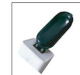
4. Insert it into a PC, or USB charger to charge the fitness band
