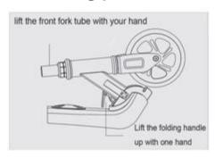
Lift the folding handle up with one hand and lift the front fork tube with the other hand and you hear a "click".
