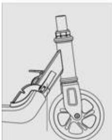
Press the folding lock firmly (the folding lock can adjust the tightness).
