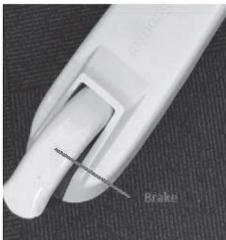
6. If you want to stop. Please use one foot to step on the rear mechanical brake. After hearing the BEEP, then continue to step on the brake until the electric kids scooter stops.
