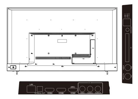
LAN(RJ45): RJ45 plug for connecting to external modem or network access equipment.
