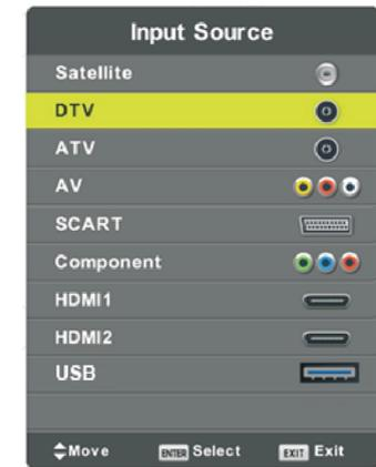
Press **INPUT** button to display the input source list
