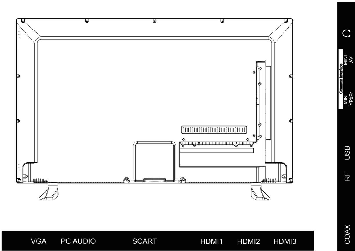
**VGA:** For PC display. Connect it to the D-Sub 15 pins analog output connector of the PC.
