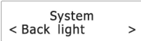
2. Press the BACKWARD or FORWARD button to cycle through the below options. The asterisk behind the option indicates the current setting.
