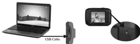
In power-off state, when the camera is connected with computer, charging begins. At this time, the charger indicator lights and it turns off when charged full. Generally, it costs 2-4 hours to charge full.
